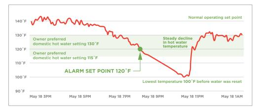
The Symmons Evolution dashboard shows the drop off in temperature of the main domestic hot water for the entire property after the domestic water heater failed. Once the burner on the water heater was reset, the domestic hot water temperature returned to normal temperature within an hour.
