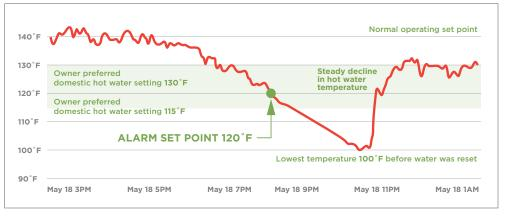
This Symmons Water Management dashboard screen shot shows the drop off in temperature of the main domestic hot water for the entire hotel after the domestic water heater failed. Once the burner on the water heater was reset, the domestic hot water temperature returned to normal temperature within an hour.
